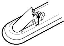
Detach the battery cover on the rear of the remote control, and insert two AAA batteries. Make sure the polarities (+ and -) are aligned correctly.
